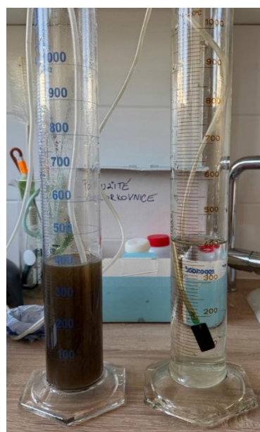
2) Metering cylinders before aeration.
